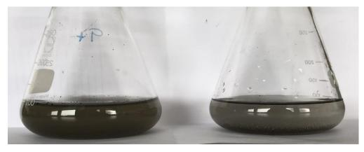
Dispersion of wood ash. 0.15% Ash. Left: Addition of 0.1% Polyaspartic acid Right: No addition. 1h after suspension.
