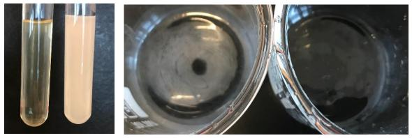
Anti-scaling test. Left picture: Sodium carbonate 3.50 g/L and 0.7 g/L mixed. Left, with addition of Polyaspartic acid (~100 ppm), right without addition of Polyaspartic acid. Right picture: Left, emptied and rinsed beaker, no addition of Polyaspartic acid. Right, emptied and rinsed beaker, with addition of Polyaspartic acid (~100 ppm)
